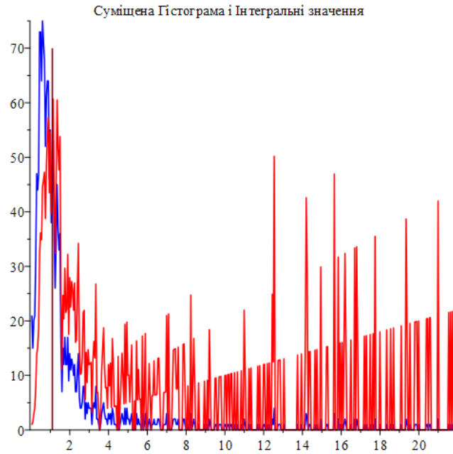
Fig. 4. Combined histogram of the frequency of emergency interruptions and their weighted contribution to SAIDI: short breaks ( t \leq m ) and long breaks ( t > m )
